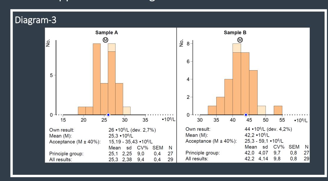
As shown in diagram-3 the results are within the normal distribution with relatively low coefficient of variations (CV%).
